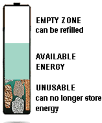
Figure 6-1: Battery charge capacity. Three imaginary sections of a battery consisting of available energy, empty zone and rock content.
