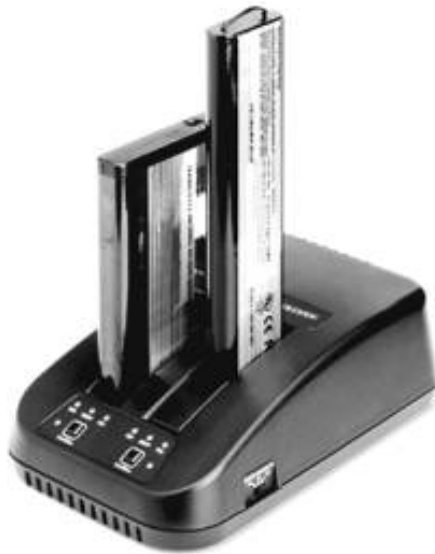
Figure 7-6: The Cadex SM2+ charger This Level 3 charger serves as charger, conditioner and quality control system. It reads the battery's true state-of-health and flags those that fall below the set target capacity. Each bay operates independently and charges NiCd, NiMH and Li ion chemistries in approximately three hours. 'Dumb' batteries can also be charged.
